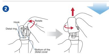
2. Keeping the gripper apart from the distal end, rotate the distal cover in the direction of the arrow as shown above until the bottom of the distal cover is removed from the hook of the distal ring to detach the distal cover.
