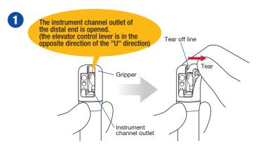
1. Hold the gripper of the distal cover and tear the top of the distal cover along the tear off line.
