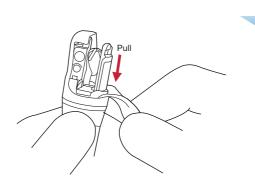
**3.** If the distal cover cannot be detached, pull the gripper toward the direction of the arrow as shown above and completely tear the distal cover from the distal end.
