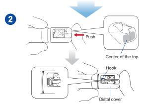
2. Put your finger onto the center on the top of the distal cover and push the top of the distal cover straight onto the distal end of the endoscope until the hook of the distal ring is completely visible within the opening of the distal cover.
