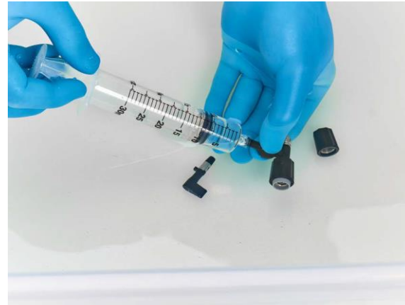
Flush the forceps/irrigation plug utilizing a 30ml syringe
