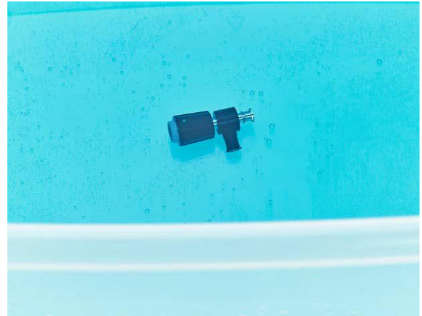
Completely immerse in detergent solution
