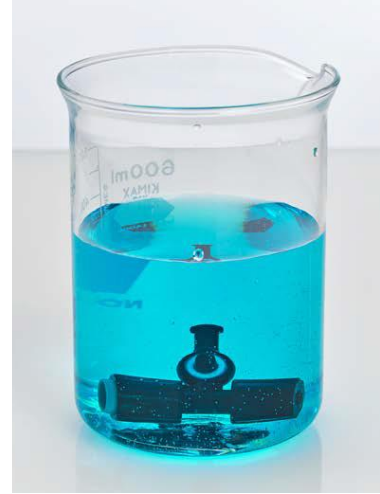
Remove MAJ-891 (top picture) or MAJ-2092 (lower picture) and immerse in detergent
