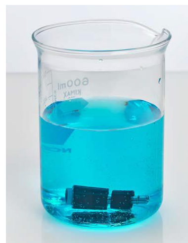
Remove MAJ-891 (top picture) or MAJ-2092 (lower picture) and immerse in detergent
