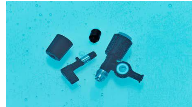
Completely immerse in detergent solution
