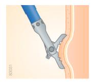
5 Double-step blade ensures sharp cutting performance and quality specimens
