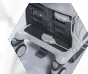
4 Active + 2 Parking Transducer Connector Ports
