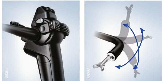
Featuring the same slim outer diameter as the conventional model\*, the ENF-VT3 is the world's first rhino-laryngo videoscope to incorporate four-direction angulation capability. The addition of 70° right/left angulation to the previously available\* 130° up/down has dramatically improved the approach to a lesion. Angulation in four-directions is possible using just one hand, allowing the other hand to simultaneously manipulate a therapeutic accessory.
