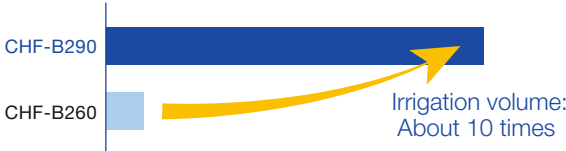
Irrigation Volume Comparison between CHF-B290 and Conventional CHF-B260 with Inserted Forceps
