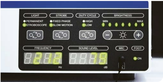
Frequency and sound pressure level are displayed on the stroboscope panel
