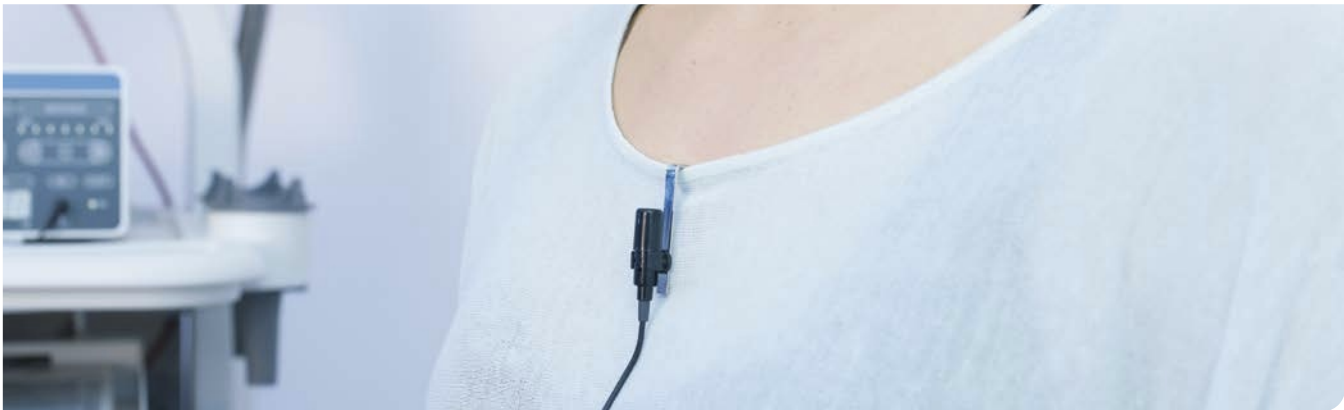
When using a clip microphone – do not place it too far from the mouth. This neck position frequently works well. Additionally, setting the microphone too close to the mouth may produce artifacts due to turbulent airflow.
